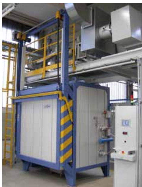
Gas-fired chamber furnace for de-binding and sintering in one process, with thermal waste gas purification system
